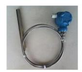
With the sensor and electronic circuit installed in connection housing, model MC20CD Gas Conduction Liquid Level Transmitter applies gas sealed in the pipe and tube to conduct liquid pressure to the pressure sensor. Avoiding direct contact between medium and pressure sensor, MC20CD can be widely used to measure high temperature and corrosive liquid. The relationship between the level and pressure is:
