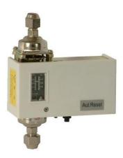
MC2040 universal differential pressure switch is a kind of delicate, flexible and convenient differential pressure switch. It is equipped with a mechanical mechanism. When the differential pressure rises or falls, the corresponding mechanism produces stretch or contraction displacement, and then push the switch action through the lever, cut off or switch on the control loop.
