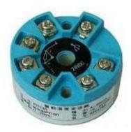
MCT80A temperature transmitter module is a temperature transmitter unit which can be on-site installed. It can be use in the junction box or fixed in the instrument box. It adopts two-wire output of  $4\sim20$ mADC (or user specified). The products have already extensively applied in the petroleum, chemistry industry, metallurgy, electric power, textile industry, food processing etc.
