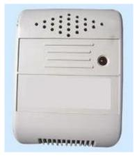
MCT80B General Wall-mounted Temperature Transmitter is a temperature transmitter which can be easily installed on the wall. It coverts the temperature value of air to standard electrical signals (e.g. 4-20ma, 0-5V etc.) for automatic control or remote data acquisition system. The products have already extensively applied in the field such as smart building telecommunication, electric power, textile industry, food processing etc.
