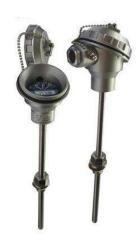
**MCT80Y Integrated Temperature Transmitter** is a kind of product can be on-site installed. It consists of thermocouple (or RTD) and temperature transmitter model, and measures the temperature of the objects. It adopts two-wire output of 4~20mADC(or user specified). The products have already extensively applied in the petroleum, chemistry industry, metallurgy, electric power, textile industry, food processing etc.
