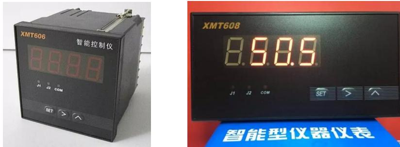
XMT6000 Universal Digital Indicator Controller integrates display, control, transmission and other functions, can accept thermocouple, thermal resistance, standard voltage or current signal, to display, control and transmit temperature, pressure level, speed, pH value and other parameters. It is widely used in thermal, chemical, electrical and mechanical engineering, and other industries. It is an ideal product for a variety of automatic control system.
