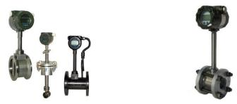
Model LUGB Vortex Flowmeter is mainly used to measure the flow of medium fluids in industrial pipelines, such as gas, liquid, steam and other media. Its characteristics are low pressure loss and no movable parts. The instrument adopts piezoelectric stress sensor with high reliability. It can work in the temperature range of - 20 ~350 ~C. There are analog standard signal and digital pulse signal output, which can be easily used in conjunction with digital systems such as computers.
