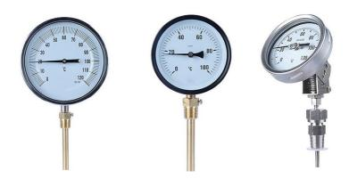
WSS series bimetal thermometer is a temperature-measuring instrument in which the differential thermal expansion of thin dissimilar metals, bonded together into a narrow strip and coiled into the shape of a helix or spiral, is used to actuate a pointer and to show the temperature value. It is also known as differential thermometer. Facilitated with all stainless steel material, it is suitable for corrosive media and environments in chemical process, petroleum and other industry field.
