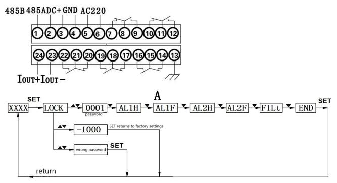
AL1H is the pull-in value of switch 1,AL1F is the release value of switch 1 AL2H is the pull-in value of switch 2, AL2F is the release value of switch 2 FILt this value is the display filter coefficient to prevent the display from jumping due to pressure fluctuation. The larger the filtering coefficient is, the more stable the display is, but the more lagged it is. 3 ~ 10 options END save exit
