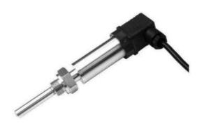
MCT80S Temperature Transmitter is a compact structure type which can be on-site installed to measure temperature and transmit corresponding signal. It consists of RTD and temperature transmitter chip that adopts two-wire output of 4~20mADC or other user specified signals for transmission. It is widely used in automatic temperature measurement and control systems such as petroleum machinery, chemical machinery, pumps and compressors, electric power, boilers, and natural gas etc.
