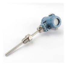
MCT80X Temperature Transmitter can be on-site installed to measure, display temperature and transmit corresponding signal to remote device. It consists of thermocouple or RTD, temperature transmitter and display module that adopts two-wire output of  $4\sim 20 \text{mADC}$  or other user specified signals for transmission. It is extensively applied in the petroleum, chemistry industry, metallurgy, electric power, textile industry, food processing etc.
