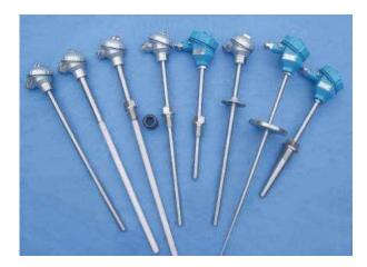
MCT80Y Temperature Transmitter is a kind of instrument which can be on-site installed to measure temperature and transmit corresponding signal. It consists of thermocouple or RTD and temperature transmitter module that adopts two-wire output of  $4\sim20\text{mADC}$  or other user specified signals for transmission. It is extensively applied in the petroleum, chemistry industry, metallurgy, electric power, textile industry, food processing etc.
