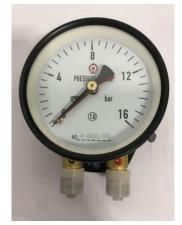
WYD-X Double Needle Duplex Pressure Gauge is mainly used for locomotive vehicles used to measure the pressure inside the hydraulic system or cylinder. It can also be used for non-corrosive, non-crystalline and solidification of the various media pressure measurement. The instrument can simultaneously measure two pressures that are the same or different (the difference between the two should not be greater than 1/3 of the upper limit of the scale range).
