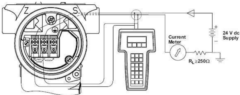
Connect the bench equipment as shown in Figure, and turn on the HART-based communicator by pressing the ON/OFF key. The communicator will search for a HART-compatible device and will indicate when the connection is made. If the communicator fails to connect, it will indicate that no device was found.
