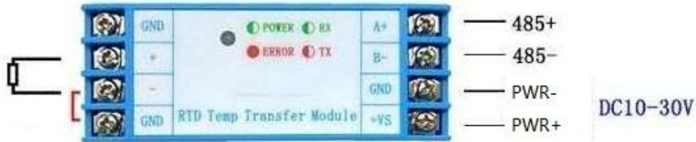
Connection of 2-wires
